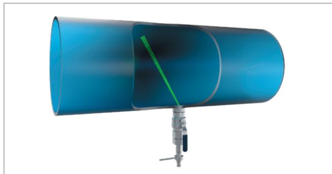
Insertion measurement in a DN400 extraction pipe
