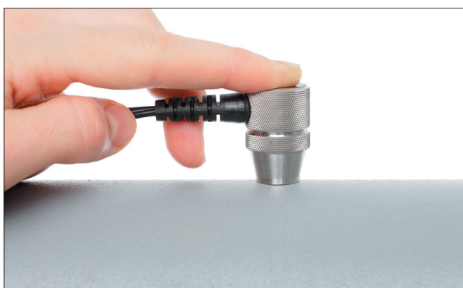
Wall thickness gauge NT in use
