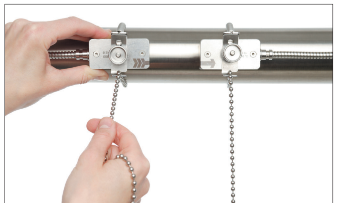
Transducers mounted using chains and clips
