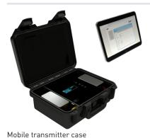
The Q-Eye Radar Portable transmitter comes in an IP67 case ready for use in harsh environments, e.g. in sewer networks. The instrument can be read out without opening the case by simply activating Wi-Fi transmission. There is no need to connect any cable for data download or configuration.
